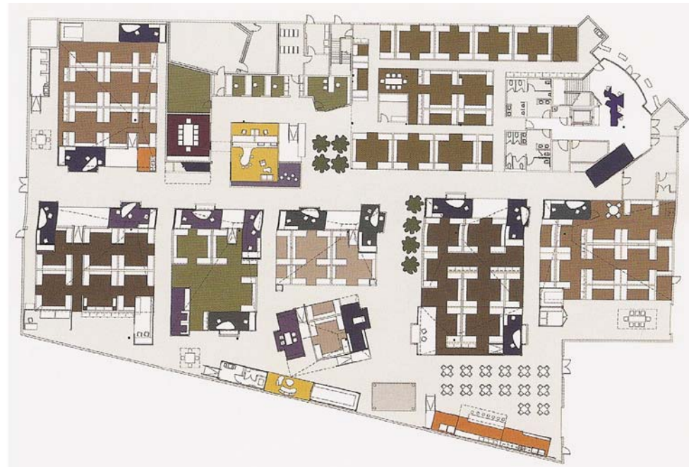
Fig 002.39: The floor configuration of [re]cycled shipping containers is used to form 'work zones'
