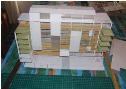
Fig 004.4.26: Corrugated panels run down the left hand side of the model, indicating more private areas such as meeting rooms. Large white panels mimic the positions of balconies on the opposite façade
