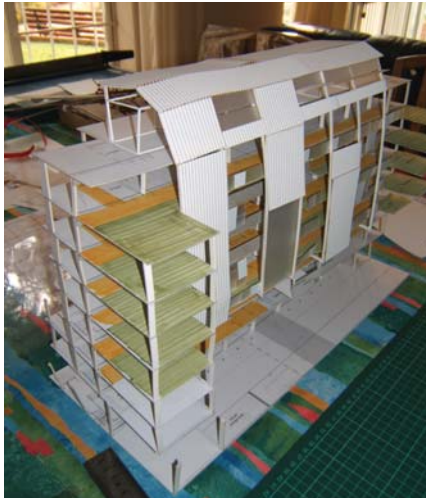
Fig 004.4.32: A photograph of the south-west corner of the concept model showing the [re]spective positions of different screening elements
