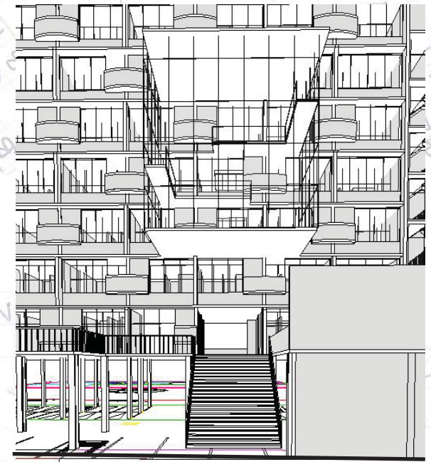
Fig 004.4.5: The new stairs form part of the new link between the German Club and 215 on Proes leading up to the new platform. The new gallery and exhibition space is contained within the glass box
