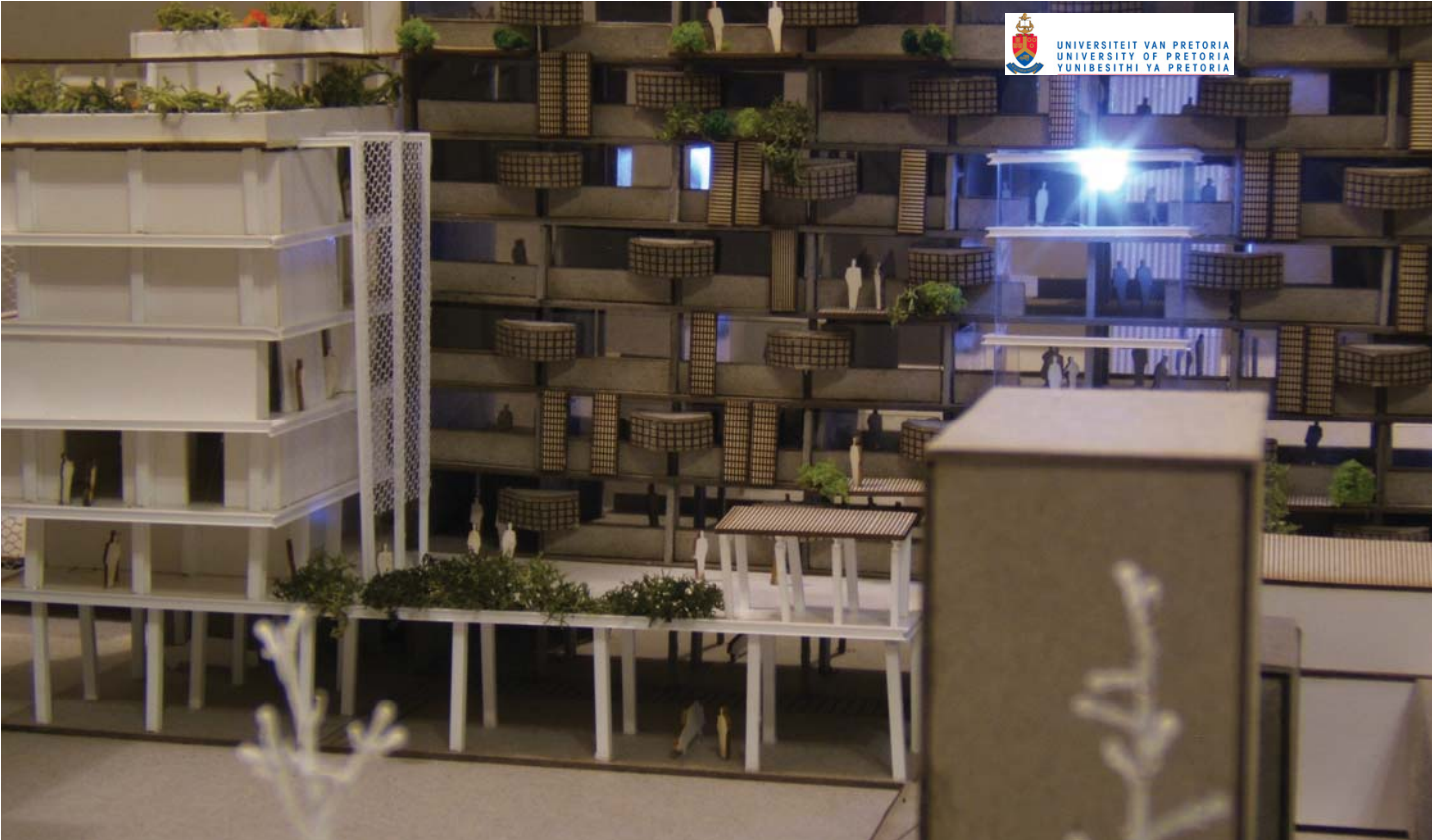
Fig 007.12: Intervention C + D are evident in this picture as is the glass gallery box. Intervention C (to the left) houses mixed-use activities. Intervention D, the platform on first floor, allows for a new public area without disturbing the existing services of the ground floor.
