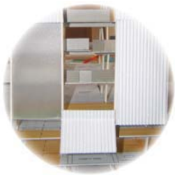
Fig 004.4.27: The translucent area [re]flects the position of the glass box on the northern façade. Screening panels are extended past the rest of the structure to indicate the entrance to the site below
