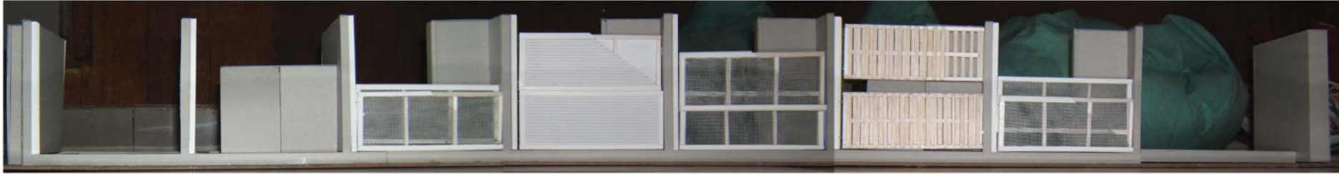
Fig 004.4.36: A sectional model through the northern façade of the building. Various screening materials are used to address the programmatic needs of the internal spaces. These screens aid in a more comfortable environment
