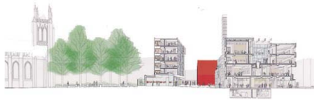
Fig 002.29: A section in perspective showing the internal configuration of the buildings as well as their proximity to one another
