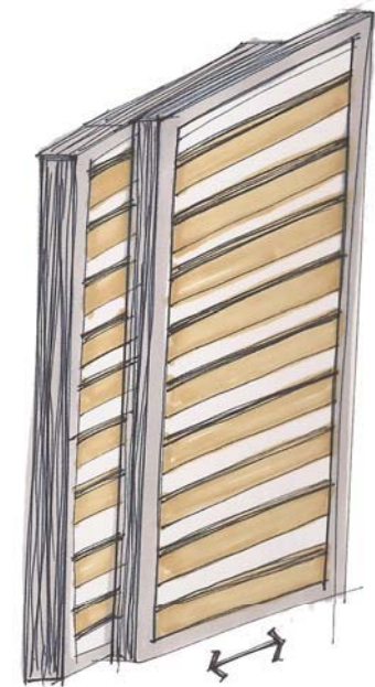
Fig 005.12: The timber screen allows for partial light infiltration as well as a degree of privacy
