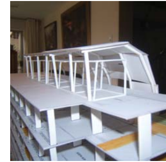
Fig 004.4.29: Residential units can be found between the trusses that wrap themselves around the building
