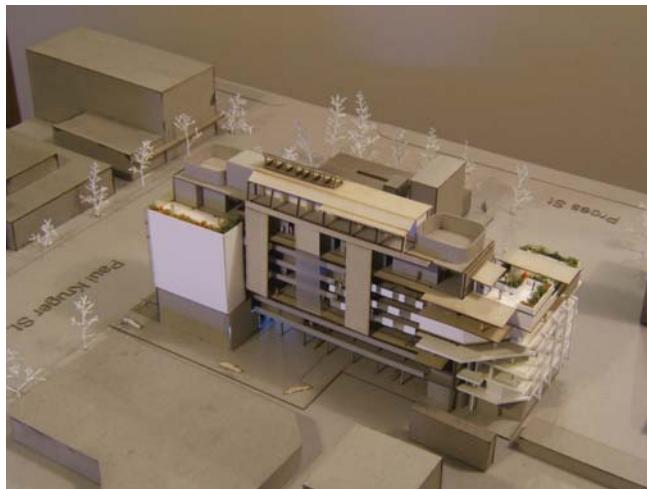
Fig 007.13: The southern façade depicts the wrapping of the various interventions around the host building. Edges of the existing are exposed
