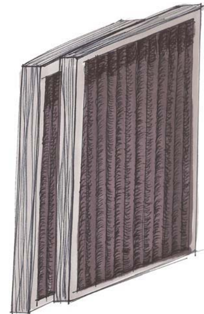
Fig 005.13: The corrugated screen allows for total light eradication and complete privacy from the outside
