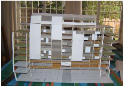
Fig 004.4.33: White panels have been included with the opaque and translucent glass. Large white panels indicate the position of balconies on the northern façade
