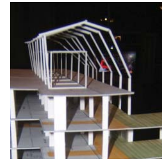
Fig 004.4.23: Trusses wrap themselves around frames which are intended for residential units
