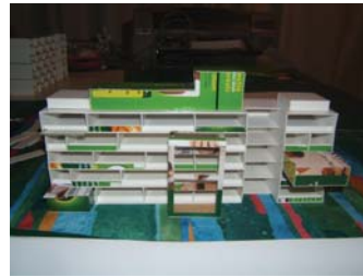
Fig 004.3.17: A “clip-on” box extending the height of three floors is incorporated on the third floor
