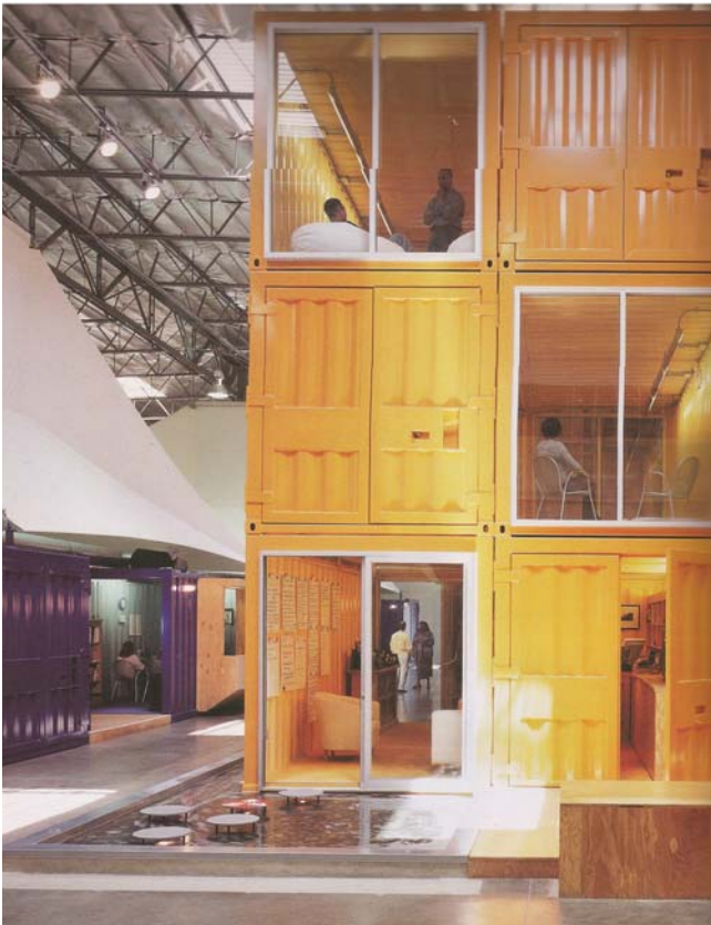
Fig 002.36: Glass sliding doors have been added to the ends of the containers to make them habitable. Further design elements such as the pond have been added for visual effect
