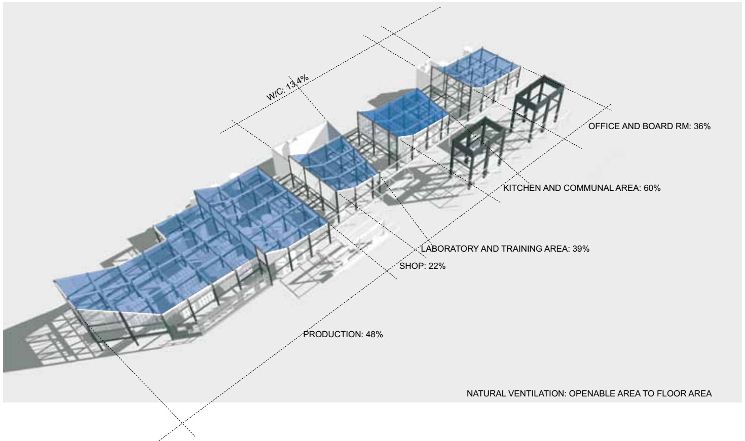
Figure 96. Pretoria West Bio-diesel plant, natural ventilation, indicating the openable area to floor area. From: Author 2010.
