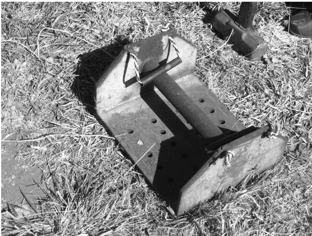
Figure 8b: The S-wave base plate. The holes are for the steel pens. It is struck on the side.
