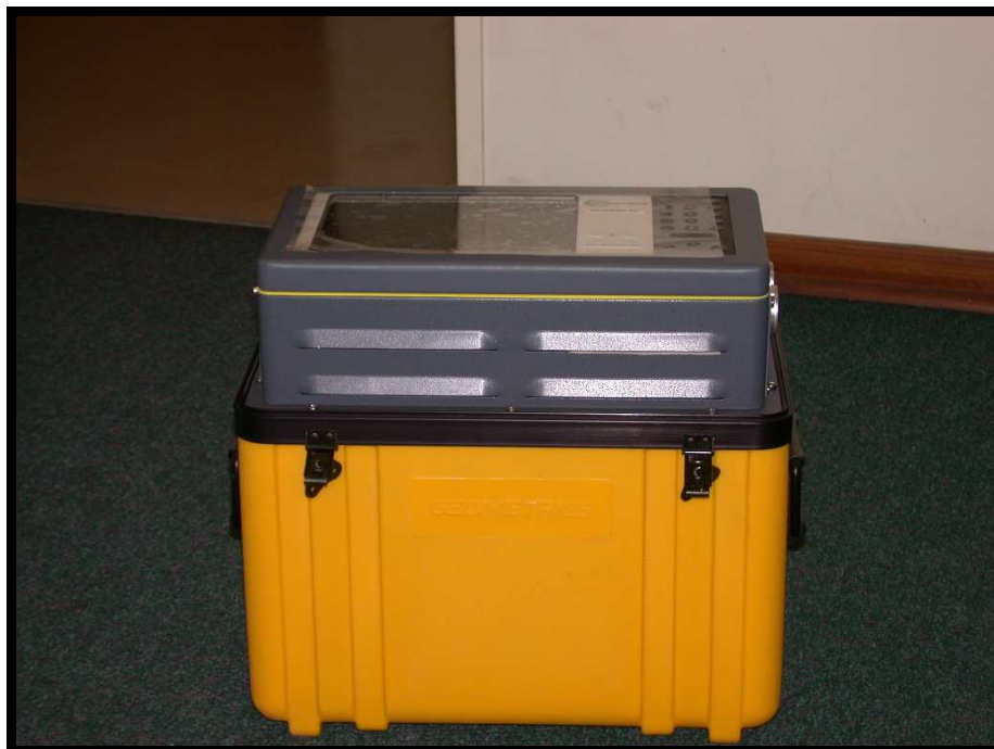
Figure 4.18: Geometrics Strataview seismograph with 24 channels that replaced the Bison Geopro seismograph, mainly because it is a floating point system.
