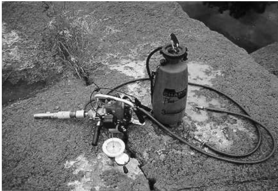
Figure 7. Diamond core drill used for taking laboratory samples.
