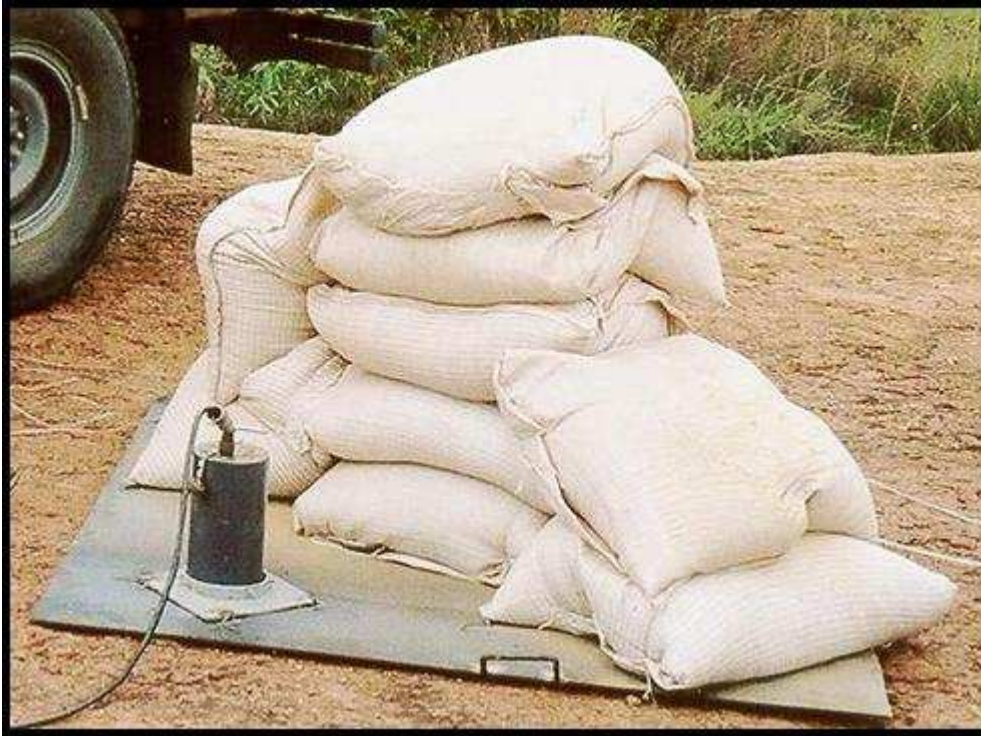
Figure 4.2: Mounting of Springheather 3-component geophone on base plate, with sand sacks to provide the weight.
