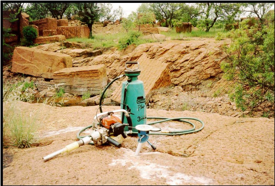
Figure 4.8: Hand held core drill used for sampling. Water with cutting oil is used to ease the drilling process.
