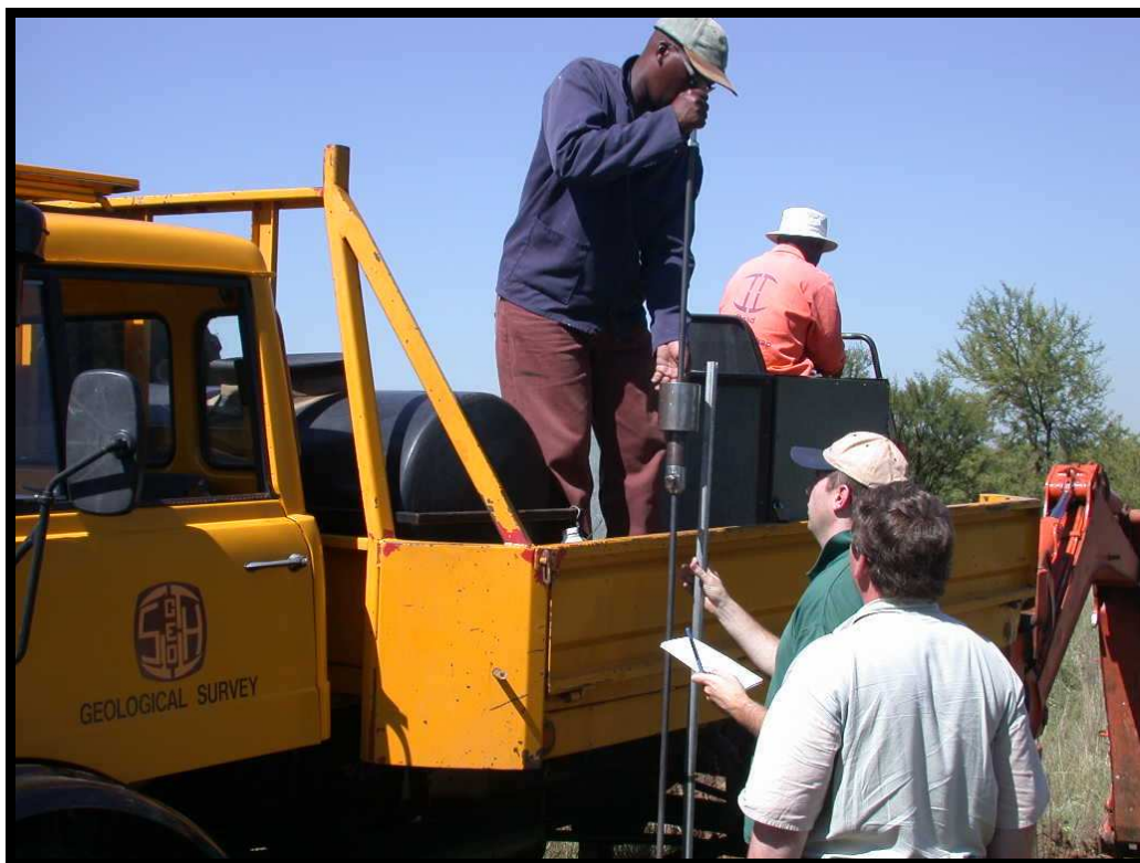
Figure 4.16: DCP test performed at each sounding position.
