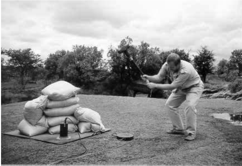
Figure 8a. Base plate, weights and seismic hammer source to generate the P-wave.
