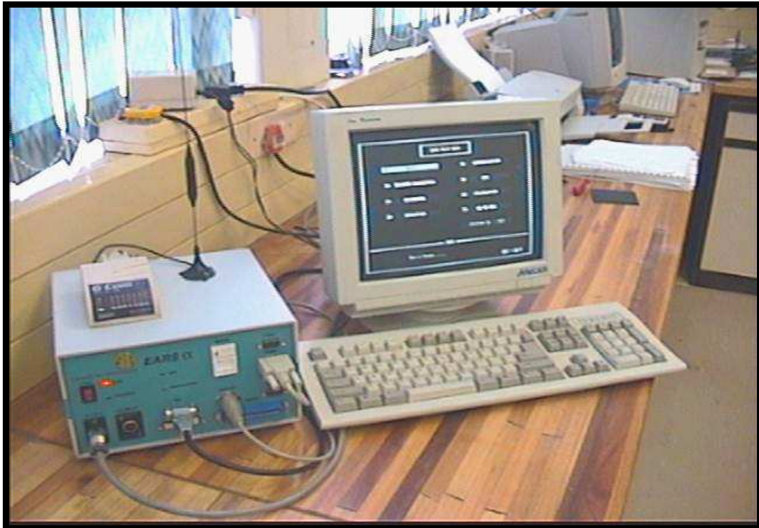
Figure 4.3: Ears- \alpha seismograph system used which is developed by the CGS.
