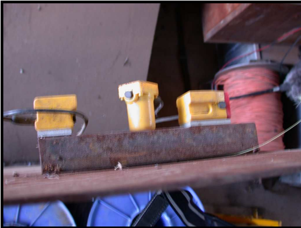
Figure 4.15: Geophones that replaced the single Springheather 3-D geophone used in the first experiment.
