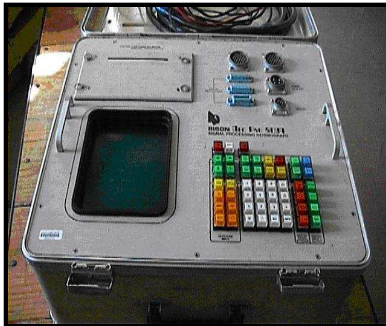
Figure 4.14: Bison seismograph that replaced ears- \alpha seismograph
