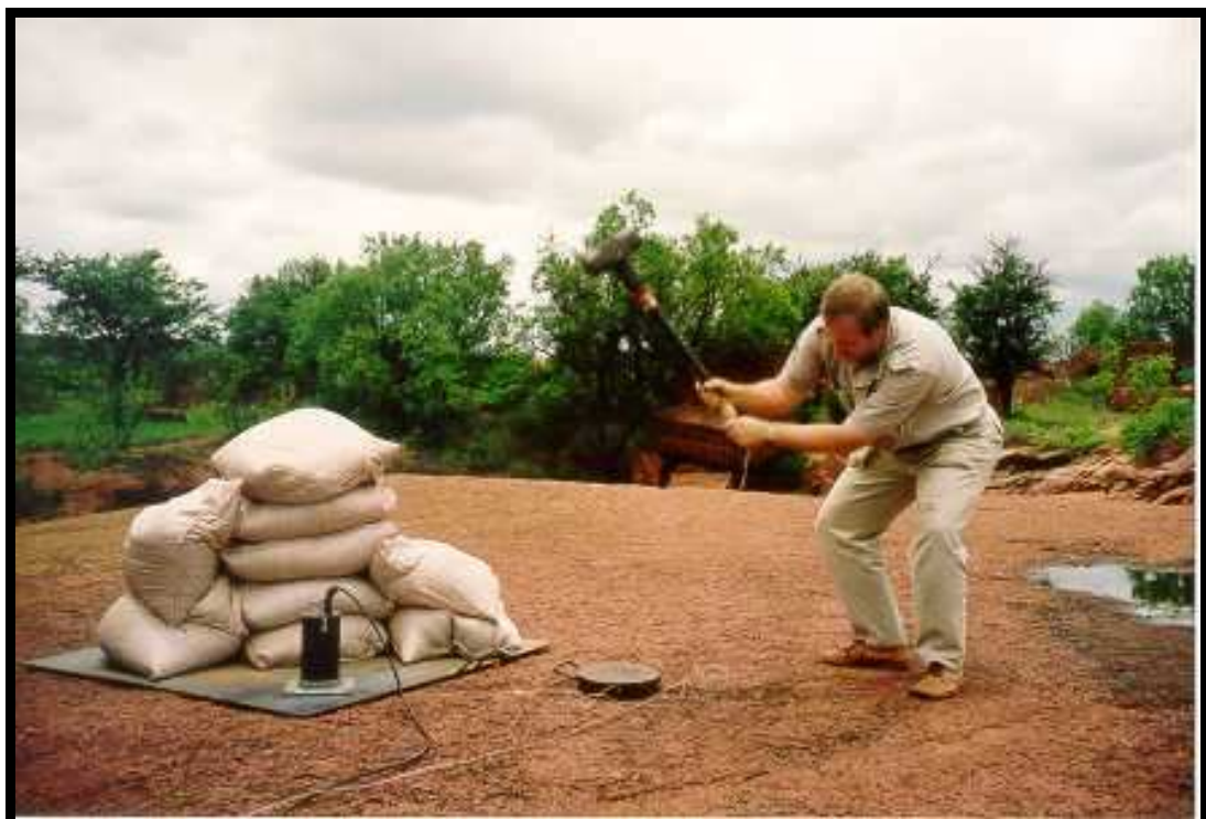
Figure 4.4: Seismic source was a sledge hammer. A hammer blow was delivered to corners of the plate.
