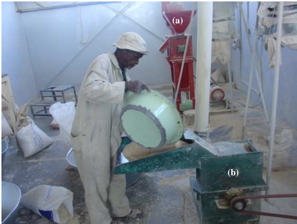
Fig. 3.1.1. PRL-type Abrasive decorticator (a) and hammer mill (b) similar to those used to produce abrasive decortication-hammer mill meal samples. Picture photographed in 2007 in Kanye, Botswana, by L Kwape.
