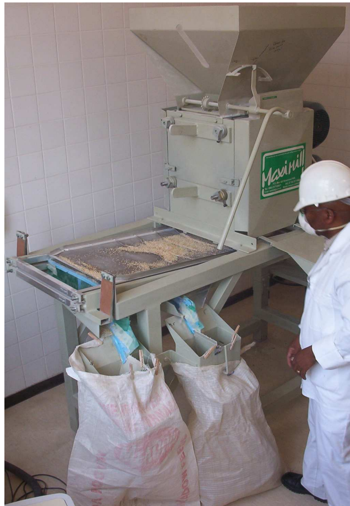
Fig. 3.1.2. Two roll roller mill used to produce roller milled meal samples. Picture photographed in 2007 at the University of Pretoria, South Africa, by L Mugode.
