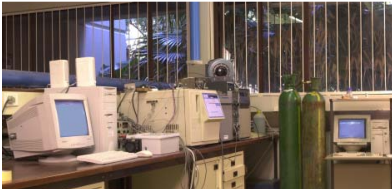
Figure 9-2: Photograph of the comprehensive two-dimensional supercritical fluid gas chromatograph.
