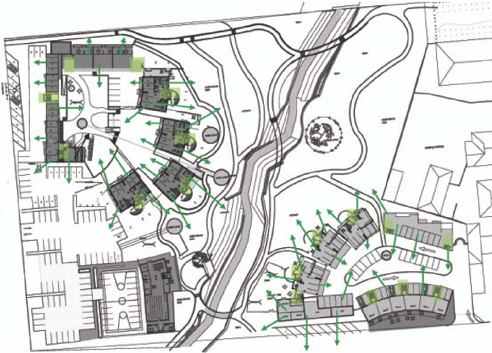
Fig 6-23 Layout of the built form: Safety - perimeter block - eyes on the street Courtyard - play area for children Opportunities for neighbors to interact
