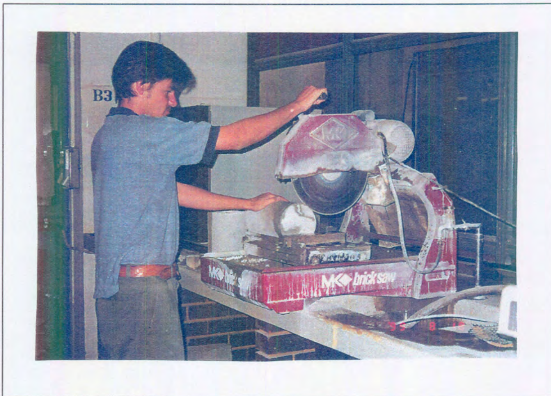
Figure 4.2: Diamond saw used for cutting of specimens
