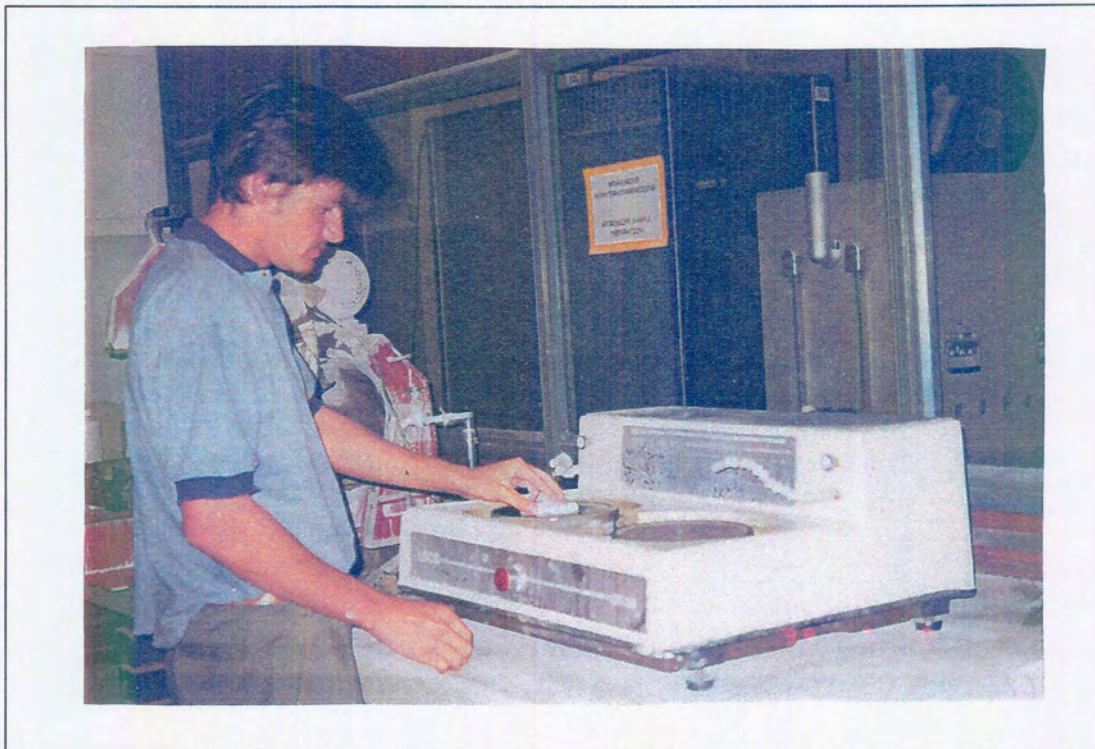
Figure 4.4: Wet grinding of test surfaces of specimens
