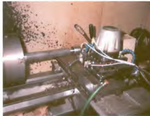
Figure 3.1 Tool changer instrumentation for the transmissibility measurement
