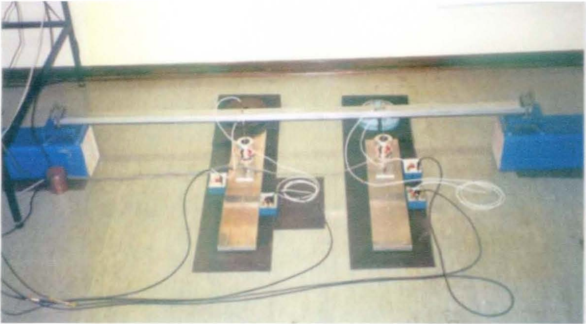
Figure E.5 – Structure-exciter attachment for hinged-hinged beam.
