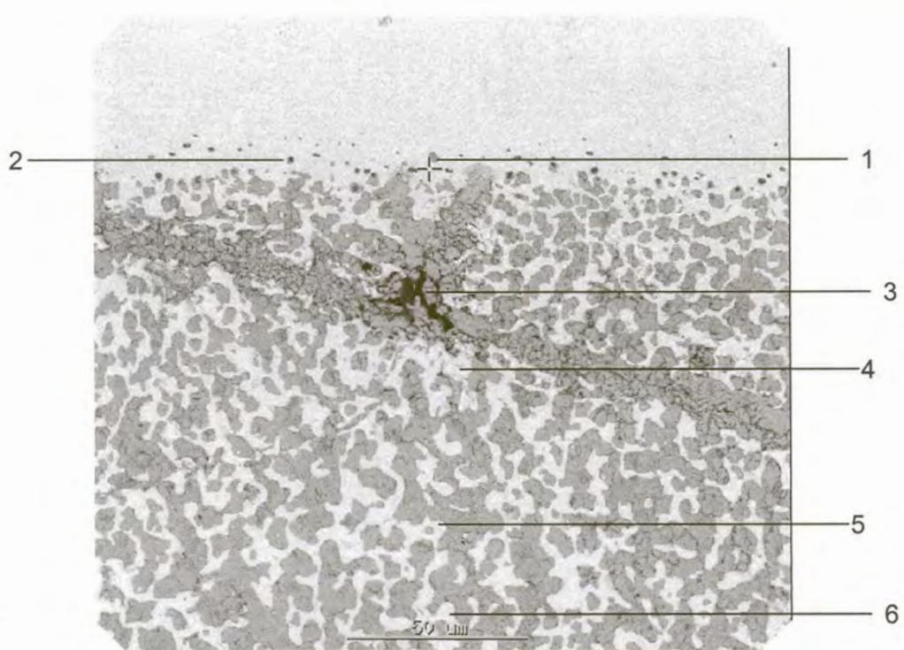
The above diagram shows the structure of scale for type 304 stainless steel reheated at  $1260^{\circ}\text{C}$  in an atmosphere with 3% excess oxygen for 6hr. The analyses of the different phases are given below.
