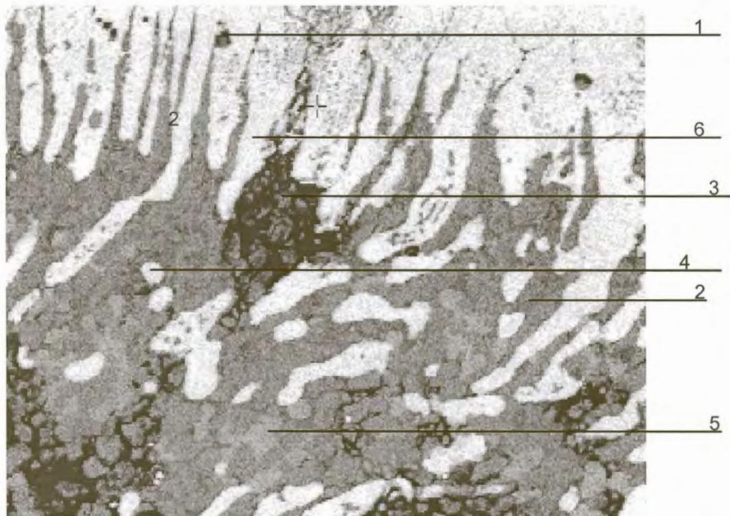
The above diagram shows the structure of scale for type 412 stainless steel reheated at  $1210^{\circ}\text{C}$  in an atmosphere with 4% excess oxygen for 6hr. The analyses of the different phases are given below.
