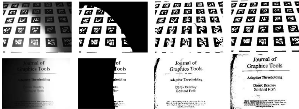
Fig. 2: Image results for each image (left) based on Otsu’s method (center-left), the Wellner algorithm (center-right) and the Integral Image algorithm (right). (Journal image from Bradley & Roth (2007).)
