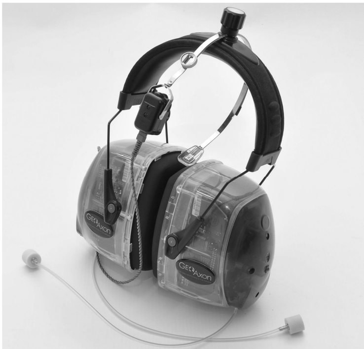
Figure 1. KUDUwave audiometer showing insert earphones, circumaural earcups housing audiometers and forehead bone conductor mounted centrally on headband
