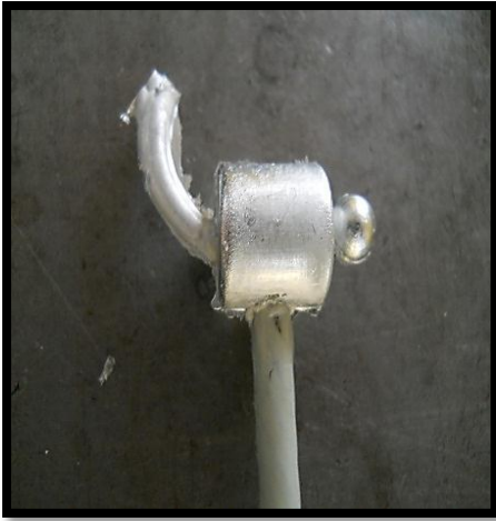
Figure 15: Uncleaned Die casted T-end
