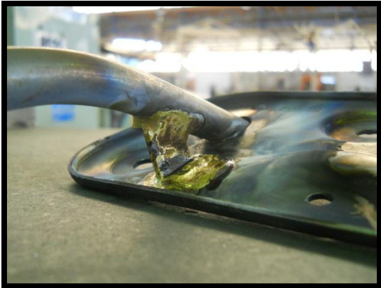
Figure 20: Brazed pipe onto plate
