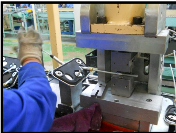
Figure 28: Second Crimping station for Screw end
