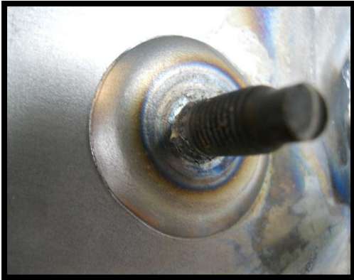
Figure 23: Spot-weld of bolt
