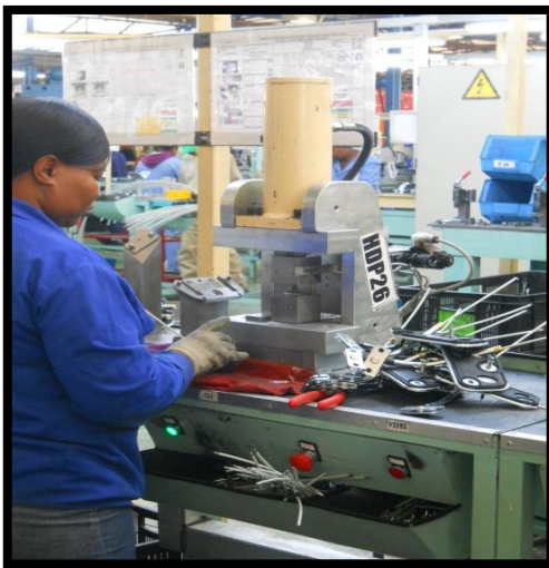
Figure 28: Second Crimping station for Screw end
