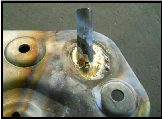
Figure 20: Brazed pipe onto plate
