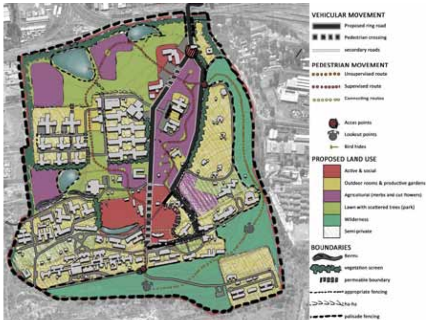
Figure 7 Proposed open space framework indicating land uses, vehicular movement, pedestrian movement and boundaries (open space framework: Van der Walt 2009).
