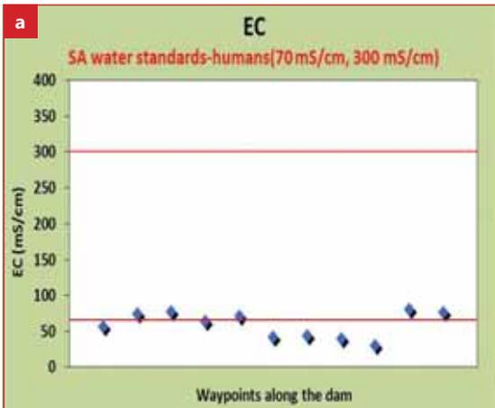
**FIG 4.1** Seasonal variation of the EC and pH in the dam: (a) EC – wet season; (b) EC – dry season; (c) pH – wet season; (d) pH – dry season. Red lines indicate the minimum and maximum allowable limit
