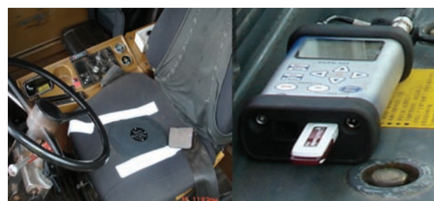
Figure 2—Dytran triaxial seat accelerometer (left) and SVAN958 HVM data acquisition system (right)
