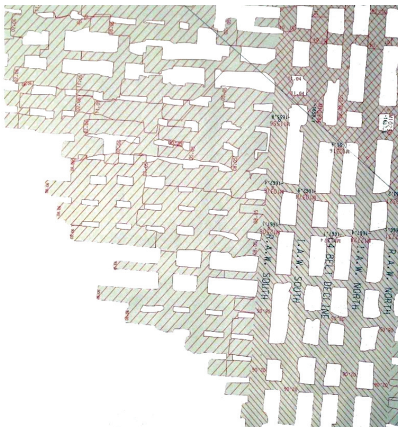
Figure 4—An example of poor pillar cutting in a platinum mine in the Bushveld Complex
