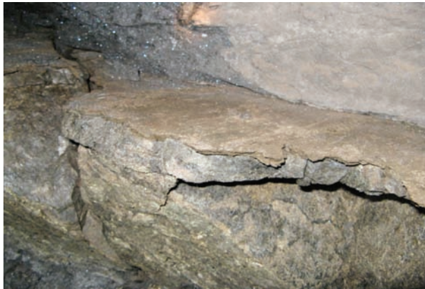
Figure 10—Presence of weak clay layers in the pillars at Wonderkop Mine. This photograph illustrates the presence of a clay layer between the LG6A chromitite and the pyroxenite below it
