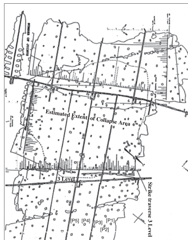
Figure 5—Extent of the collapse (dotted line) at No 6 Shaft, Bafokeng North mine
