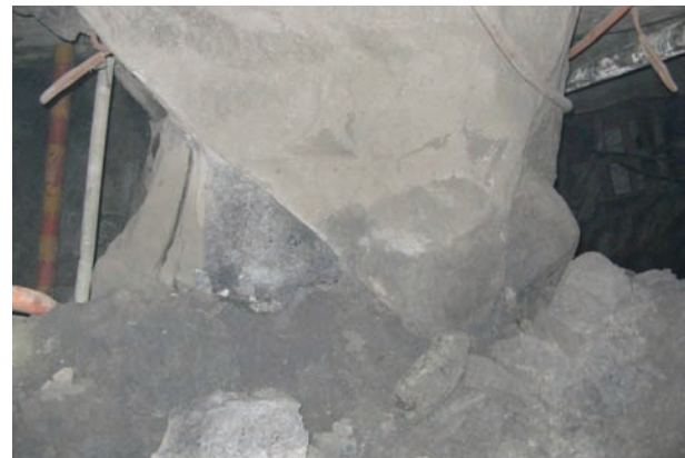
Figure 20—An example of a pillar that contains a single joint dipping at almost 45° through the pillar. This joint will have to be modelled explicitly if the behaviour of this pillar is to be correctly simulated by a numerical modelling code
