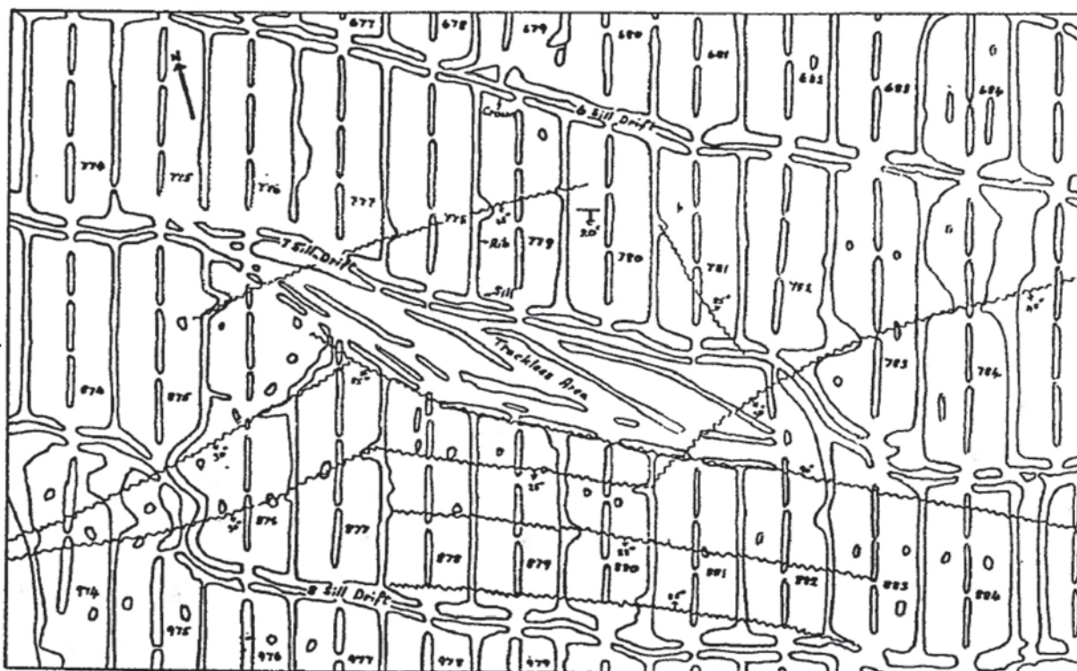
Figure 7—Typical layout of a mine in the Elliot Lake district (after Hedley, Roxburgh and Muppalaneni 24 )
