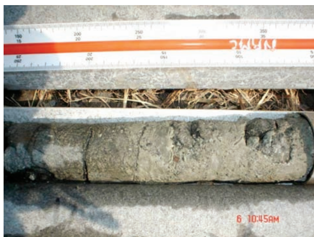
Figure 11—Presence of weak clay layers in proximity to the LG6/LG6A chromitite reefs at Wonderkop Mine
