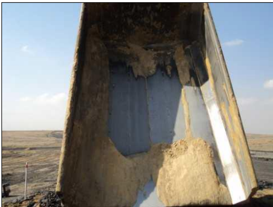
Figure 3: Example of Severe Carry-back Problem.
