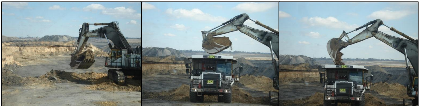
Figure 7: Loading of CAT 773 – 502 in Overburden Removal Process.
