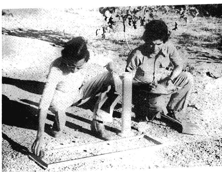
FIGURE 10.4 - TECHNICIANS MEASURING RUT DEPTH AND GRAVEL LOOSENESS ON AN UNPAVED ROAD
