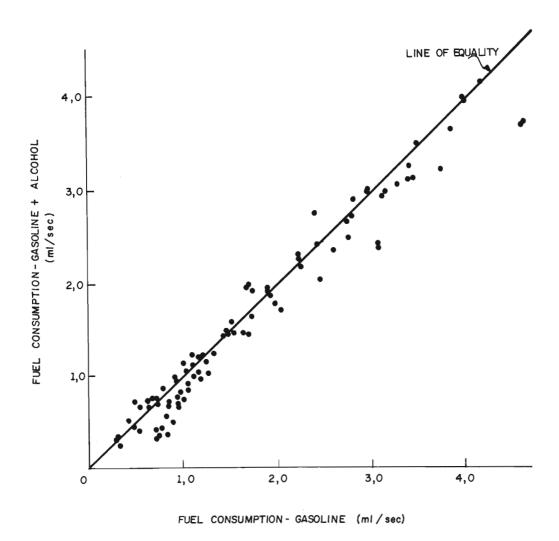
FIGURE 7.3 - GRAPH COMPARING THE CONSUMPTION OF PURE GASOLINE WITH THAT OF GASOLINE + ALCOHOL (UTILITIES).
