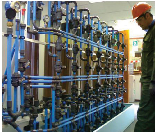
Figure 7: ion-exchange columns in pilot plant (DOYLE, Dr Richard, 2009)
