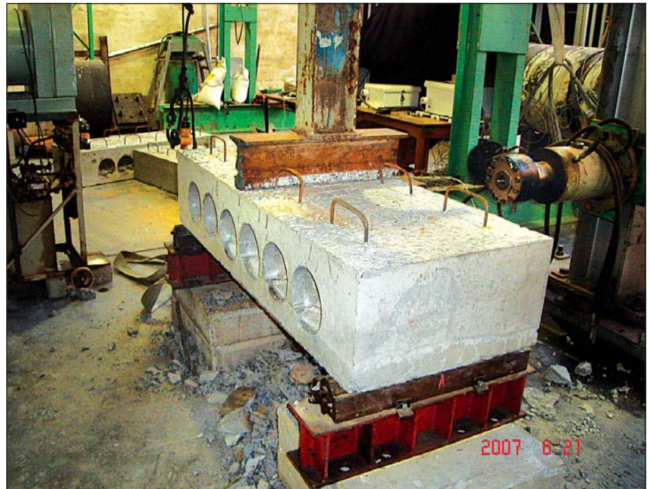
Photo 1 Experimental setup of an SFV sample at the University of Pretoria (UP 2007)
