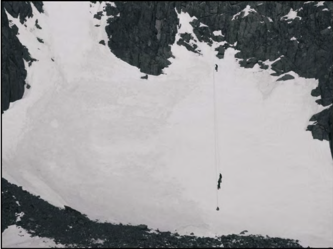
Figure 4: Releasing clasts from approximately 5m below the top of the firn field. Note the firn (ice) was hard enough to use crampons. Note the people for scale.
