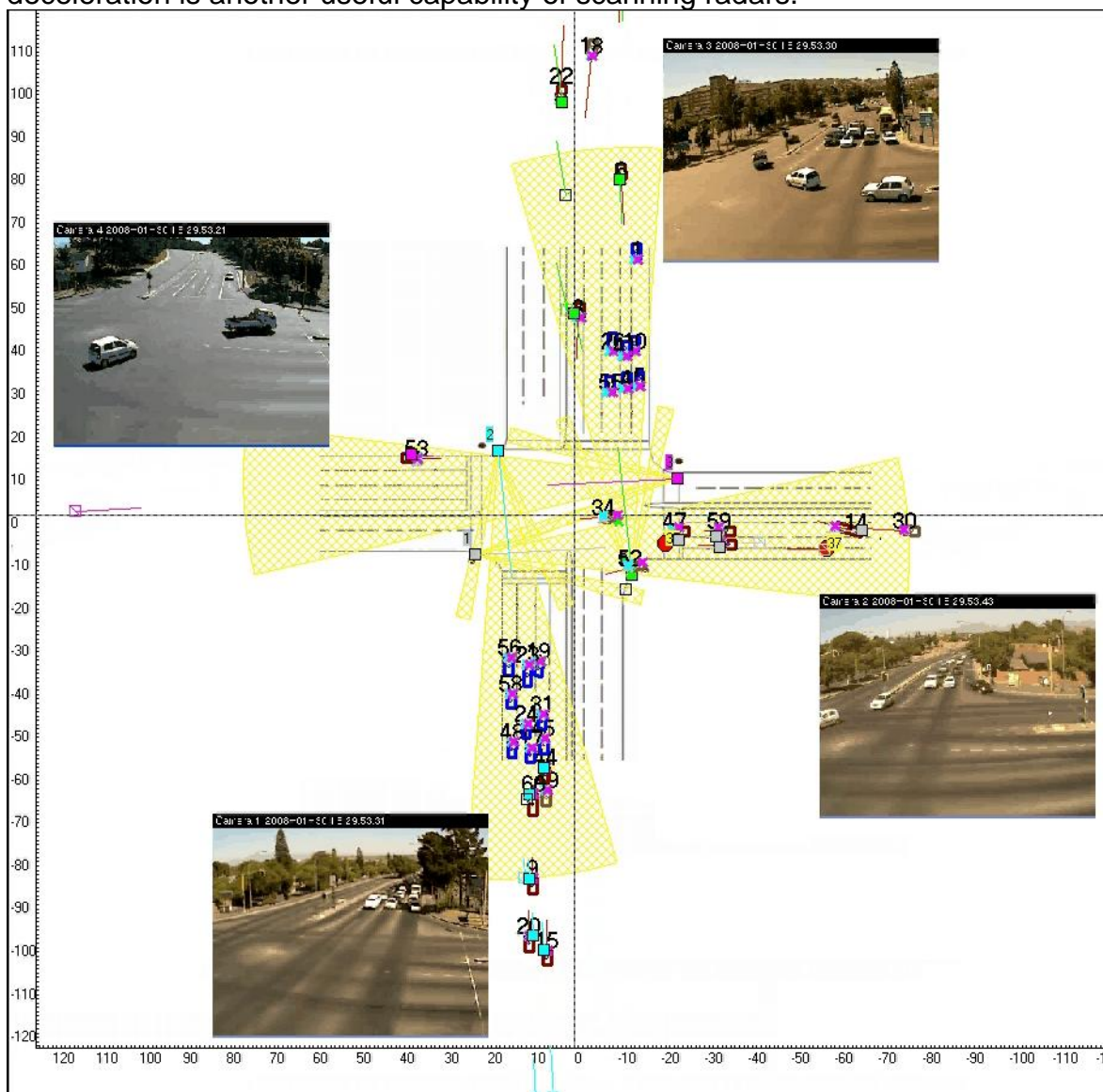
Figure 2: One 50ms measurement frame at an intersection in Cape Town. Each tracked target (vehicle) is assigned an ID shown next to each square. The ID is maintained as long as the vehicle is within 240m from the intersection. The velocity and vehicle length is known for each vehicle and each instance.
