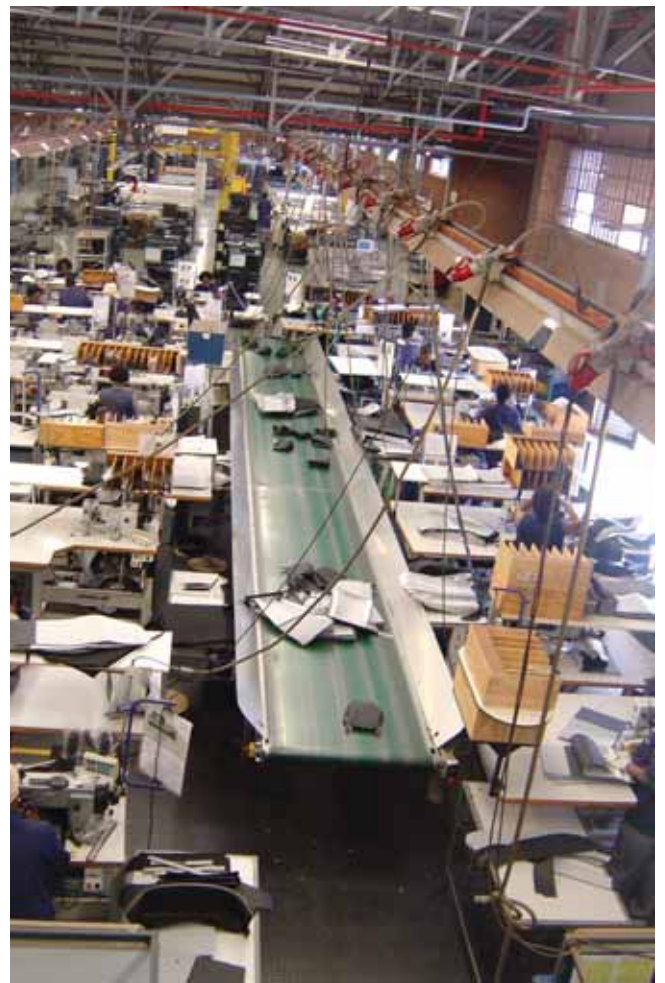
This is “stand-up-sewing”: The tables were height-adjustable, and the conveyor-belt decreased the need for reaching. Note the racks for parts above the machines. The musculoskeletal strain on the upper body here was much less than on the “sit-down-sewing line”
