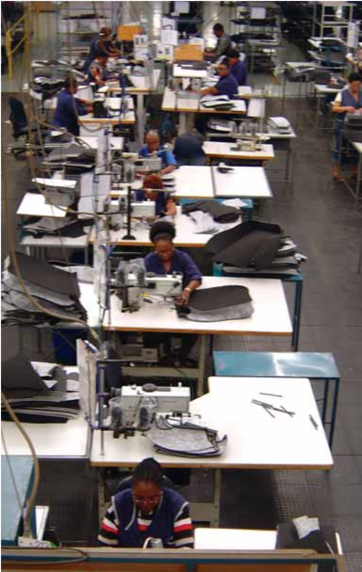
This is “sit-down-sewing”: The tables were not height-adjustable, and a lot of reaching was involved to pass the covers on to each other
