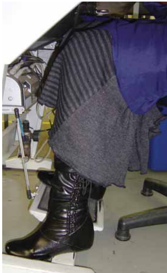
A common problem: Tall tibias caused the knee caps to bump into the belly of the sewing machine underneath the table. To prevent this discomfort, the operator will sit farther from the machine – as the pedals are fixed – causing her to reach forward. This posture change leads to back and upper-extremity muscle discomfort
