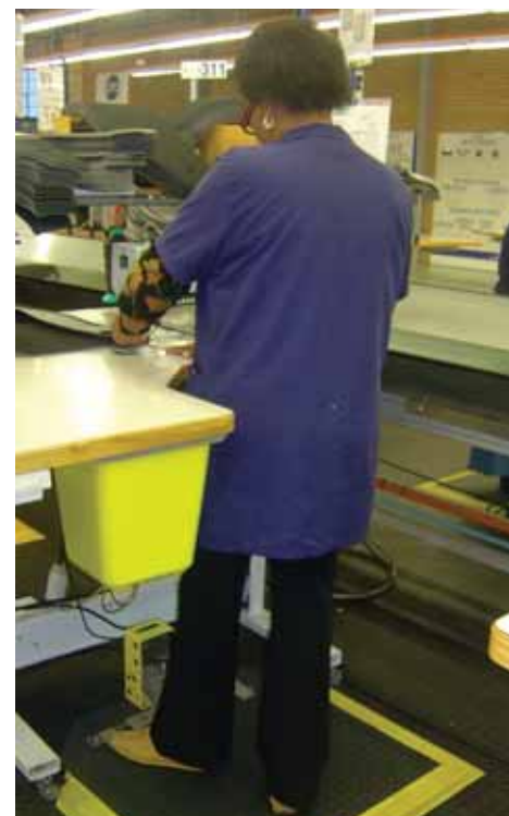
This table was not height-adjustable. The preferred height for precision work is elbow height.
