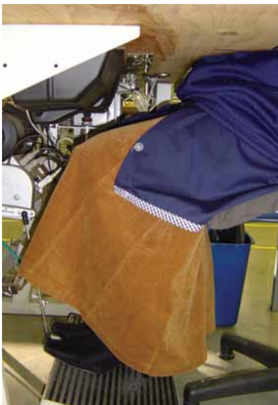
The solution for the leg space problem underneath the table was to ask the maintenance team to increase the table height. This would enable the operator to sit closer to the table, but might also lead to upper shoulder muscle spasm
