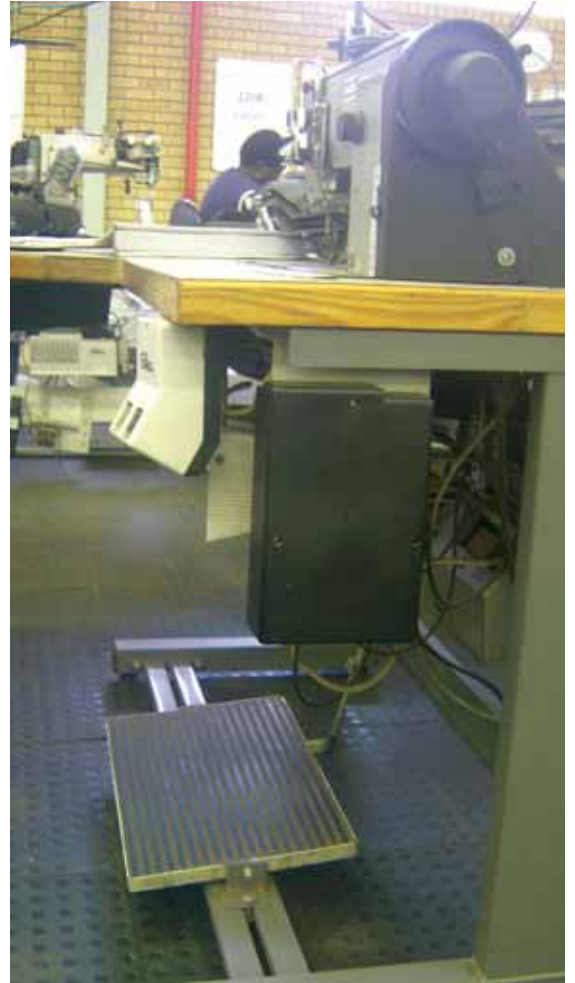
The pedals were all fixed onto the tables. The position of this pedal caused the operator to sit far from the machine and lean forward to sew. This would lead to increased strain on the upper extremities and back muscles
