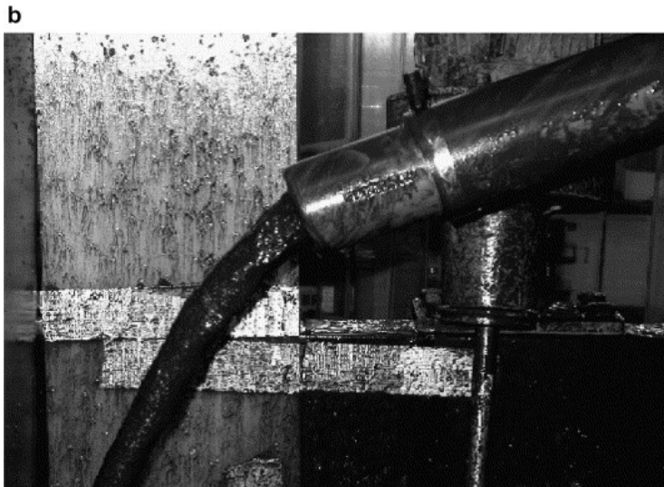
Fig. 2. (a) Spray and (b) rope discharge at the underflow.
