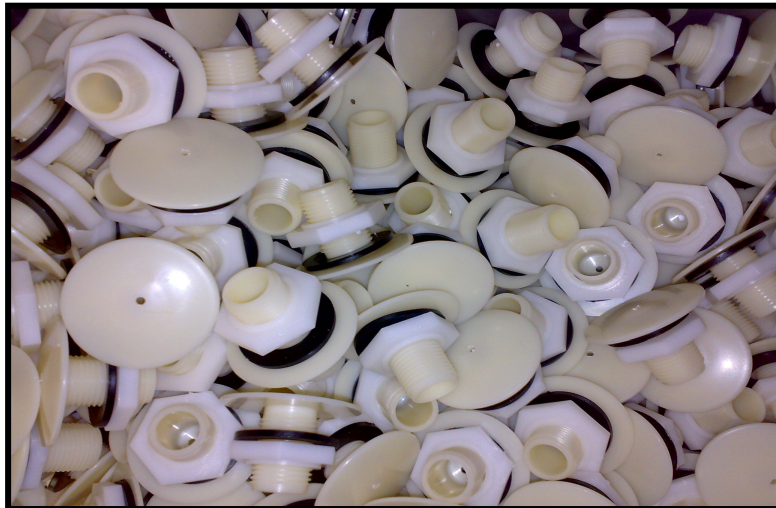
Figure 3: Flanges that will be glued to the filter candles during the assembling process. 2009. Photo taken by author
