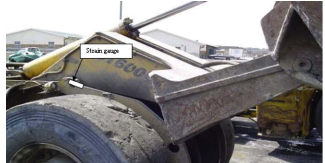
Fig. 7. Strain gauge position on boom (channel 3).
