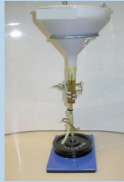
Baermann apparatus set up to examine faecal samples for lungworm larvae. A sieve and some gauze are positioned in the funnel, onto which the faeces and some water are placed and left for 24 to 48 hours. The larvae migrate through the gauze and settle in the neck of the funnel. The water is then drained out of the tube at the bottom and the sediment examined microscopically for the presence of first-stage larvae
