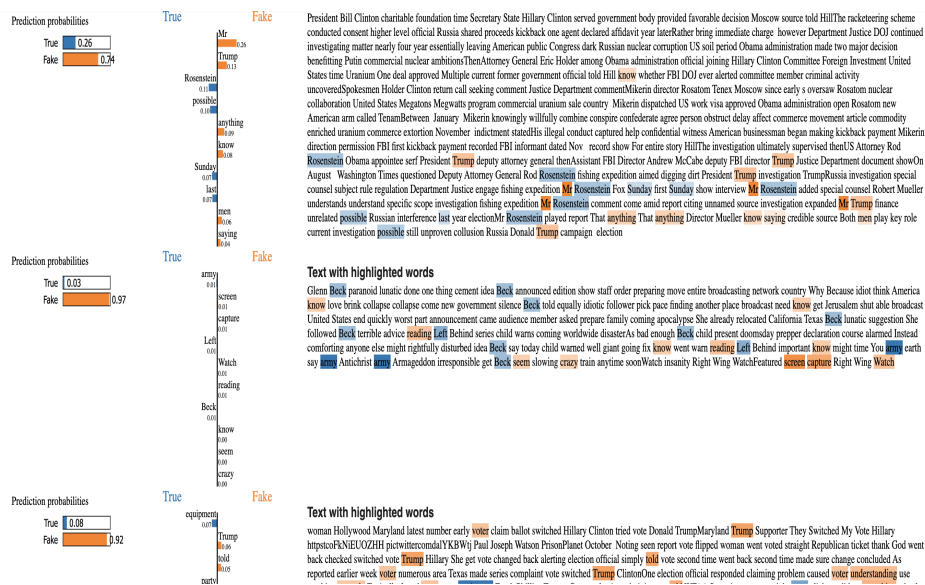
Figure 6.43: Output of using SP-LIME with Prototypical examples to explain and indicate prevalent words for Fake news class
