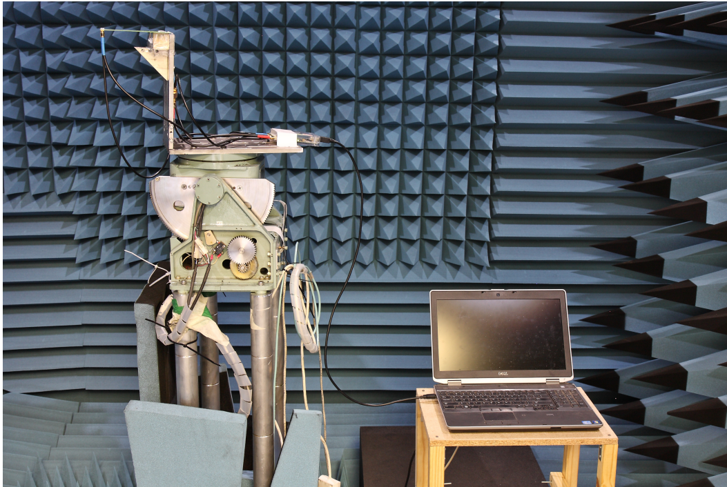
Figure 5.3. Photograph of the radar antennas mounted on the positioner in the anechoic chamber. The SDR and computer running the radar code can also be seen. (Photo credit: Prof. W. P. du Plessis)
