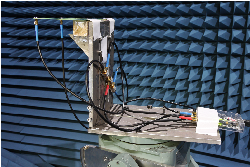
Figure 5.4. A close-up photo of the radar antennas mounted on the positioner. The SDR and power dividers can also be seen. (Photo credit: Prof. W. P. du Plessis)
