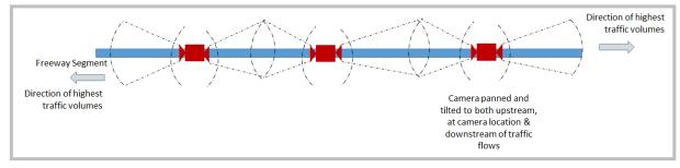
Figure 6: Roaming view camera surveillance
