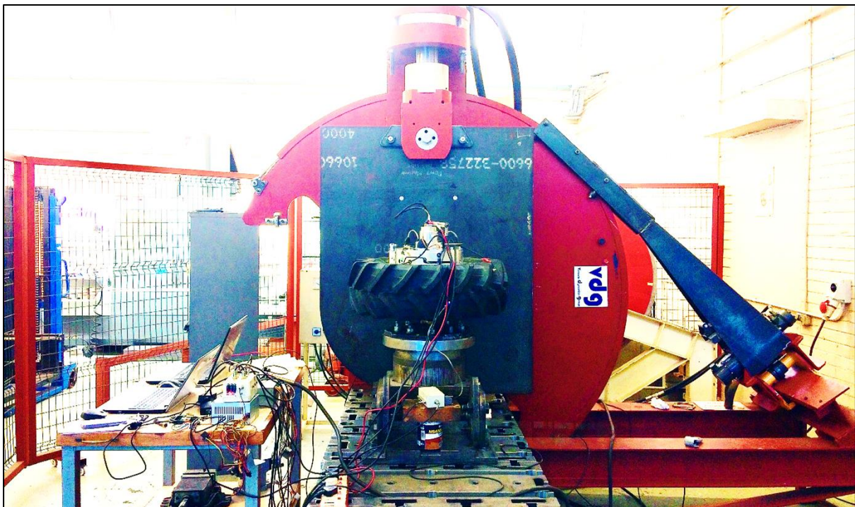
Figure 46- Test Setup on Static Tyre Test Rig
