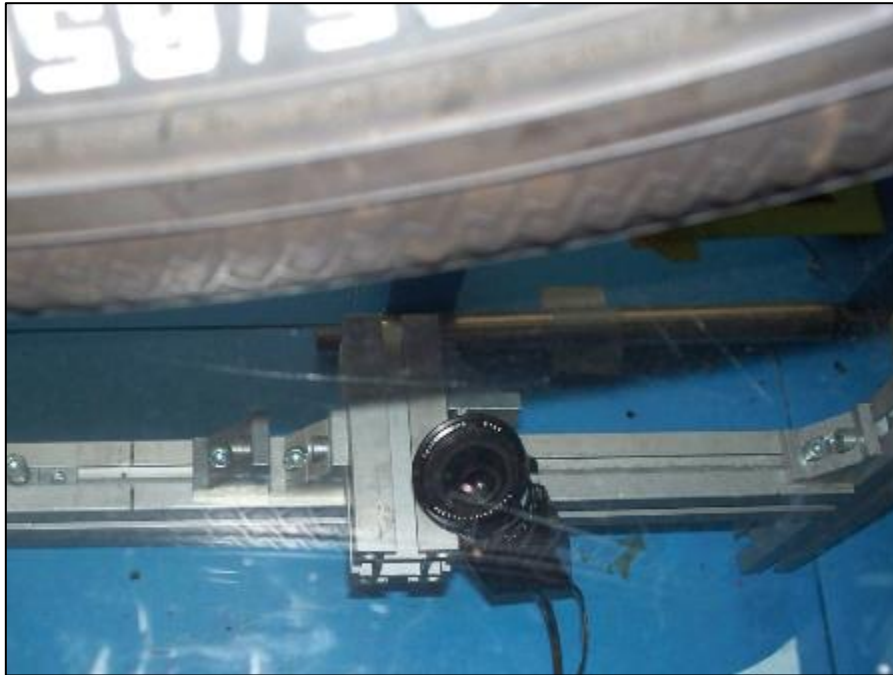
Figure 2- Tyre contact patch test rig (Ivanov, 2010)
