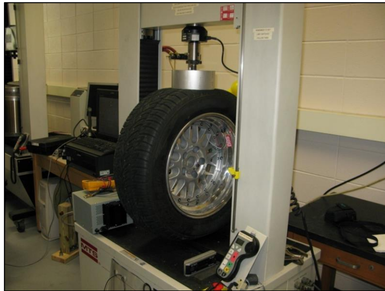
Figure 8- Deflecting Tyre in Vertical Direction (Green, 2011)
