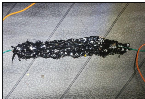
Figure 5- CTPE Prototype Strain Sensor Showing One Sensor (Ruggeri and Vecchiattini, 2018)
