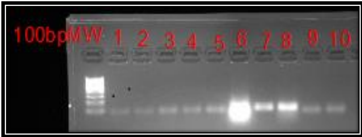
Figure 3.7: Specificity of qPCR amplification. A) Melting curves of the ten genes selected for constitutive expression validation showing a single melting peak for each product (each including two biological replicates and a no template control). B) Agarose gel (2%) showing qPCR amplicons generated by specific amplification of the 10 selected stably expressed genes. Lanes 1-10 represent genes with the accession number: XM_758090.1; XM_757859.1; XM_758360.1; XM_758301.1; XM_758834.1; XM_759300.1; XM_759535.1:XM_759942.1; XM_760594.1; XM_760631.1 respectively.
