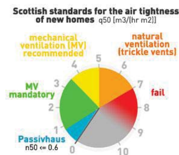
Figure 1 Air tightness requirements
