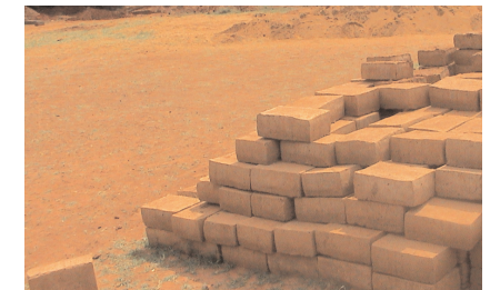
Fig. 2.4.6.2.4.2 Compacted earth blocks
