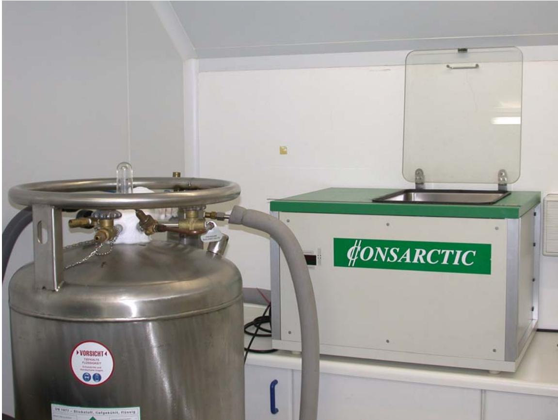
Fig. 4.4. The cryopreservation chamber and liquid nitrogen storage tank that was used to perform the controlled freezing of the collagen-GAG co-precipitates. An initial temperature of 20°C was lowered at a controlled rate of 0.92°C/min to reach a final temperature of -40°C.
