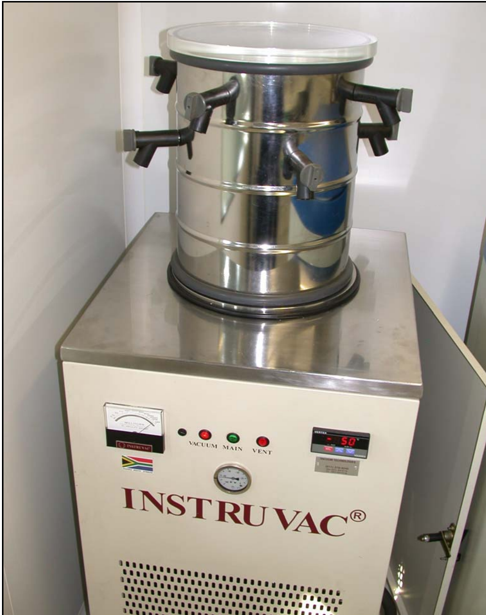
Fig. 4.5. The INSTRUVAC ® lyophilization chamber that was used for the sublimation of ice crystals from the prepared collagen-GAG scaffolds. The prepared scaffolds were lyophilized for at least 17 hours.
