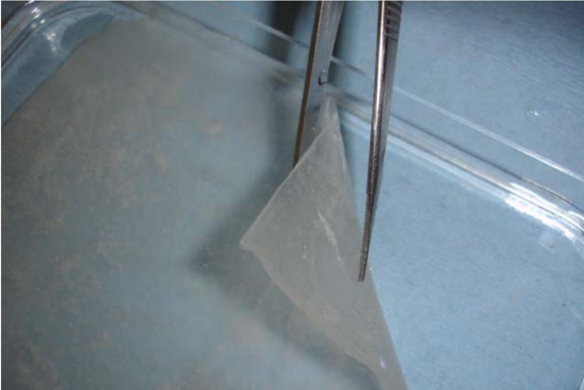
Fig. 5.8. This photo demonstrates the crosslinked artificial skin which consists of an epidermal portion (the exposed inferior surface) and a dermal portion (superior).
