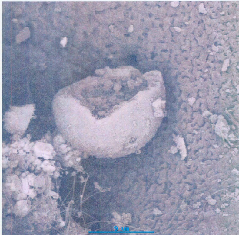
Plate 5. c Micrographs for the residue from the combustion of Sb_6O_{13} - 20%Si (type 4) in lead tube.
