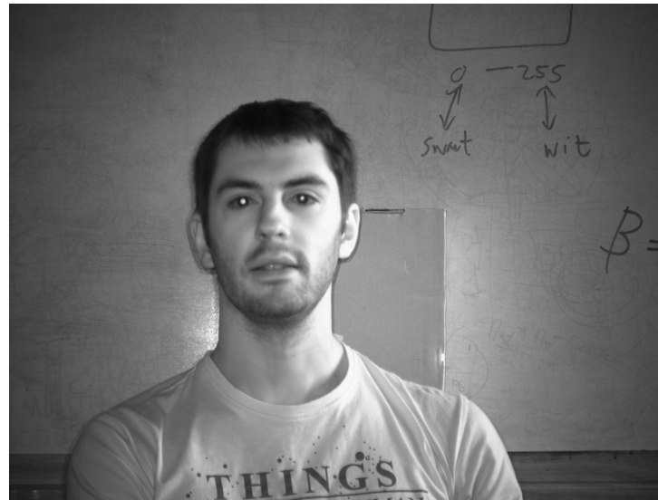
Figure 5.6: The bright pupil image as produced by on-center illumination from 780nm NIR LEDs.
