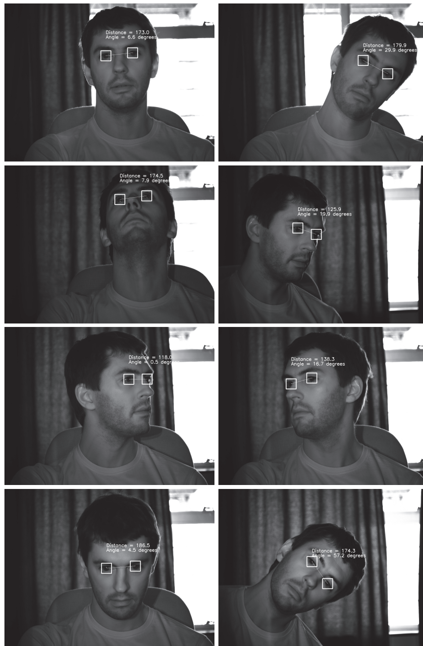
Figure 5.12: Eye detection results for a subject without wearing glasses, for various head poses, some of which caused significant occlusion. In each example image the distance between the detected eyes as well as the angle between the eyes (with respect to the horizontal plane) are also given.
