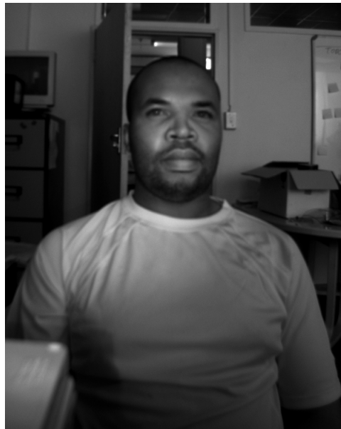
Figure 5.3: An example image of an unsuccessful attempt to obtain the bright pupil effect with 850nm NIR LEDs in a subject from African decent.
