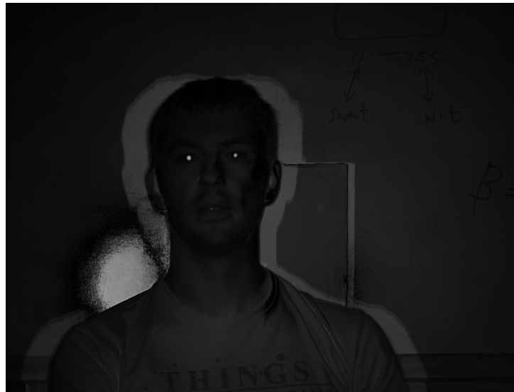
Figure 5.8: The resulting difference image from subtracting the dark pupil image (Figure 5.7) from the bright pupil image (Figure 5.6).
