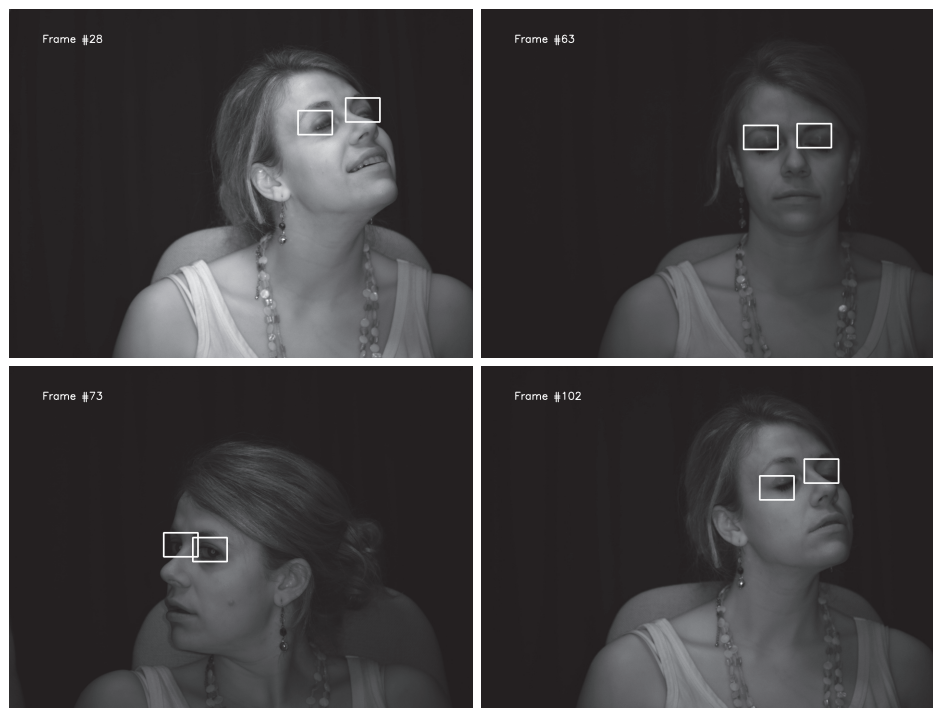
Figure 5.18: Four eye tracking example images of a Caucasian female for eye occlusions due to sideways head rotation and blinking. For these examples, it is apparent that the system could handle these types of eye occlusions.
