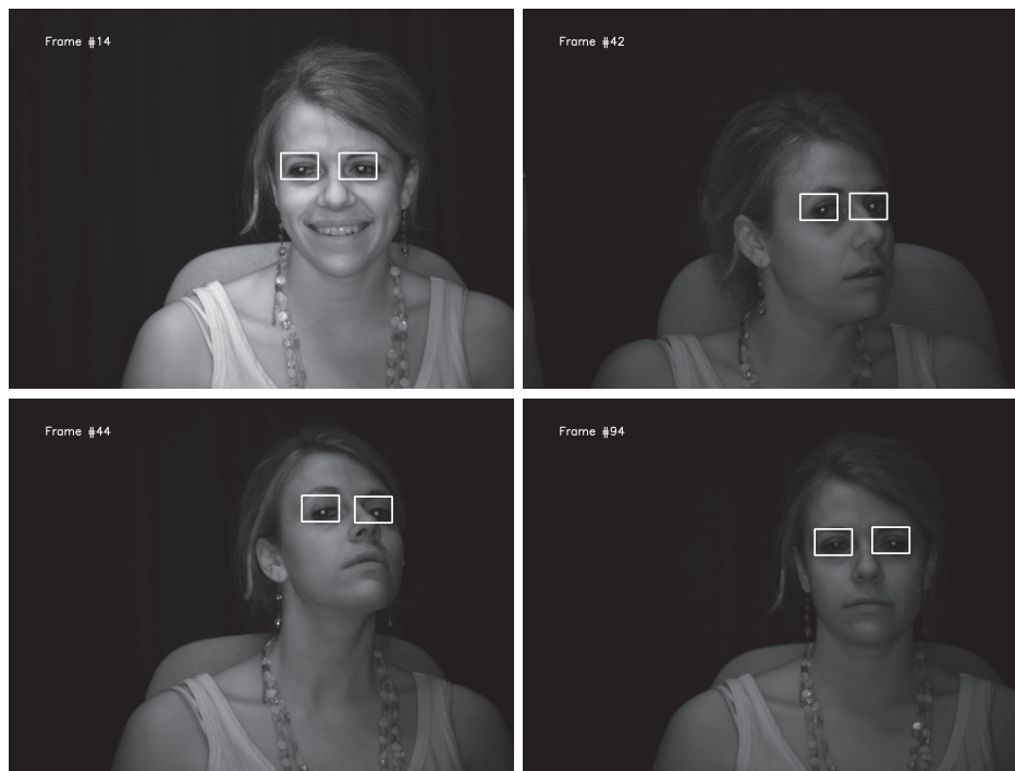
Figure 5.17: A few consecutive eye tracking example images of a Caucasian female under reasonable head movements. The frame numbers in the sequence are also shown in each image.
