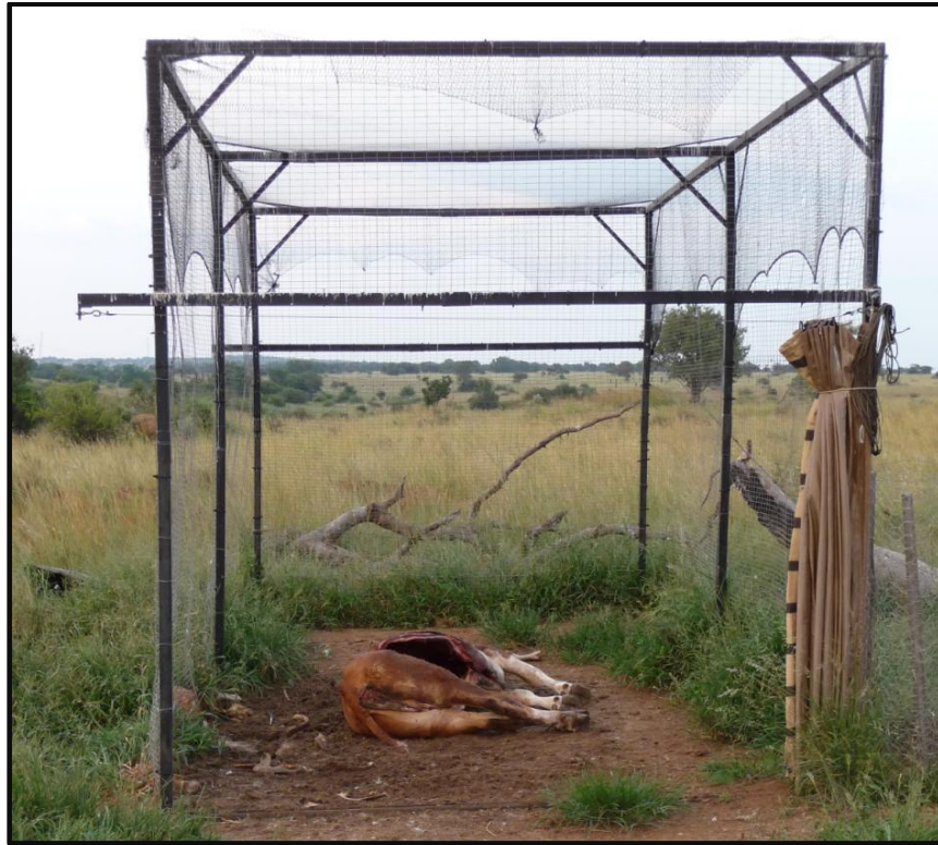
Figure 3.3. Photograph of a heifer carcass inside the walk-in capture cage at Mankwe Wildlife Reserve. The curtain was closed by pulling a cable attached to the bottom corner after the target vulture(s) had entered the cage.
