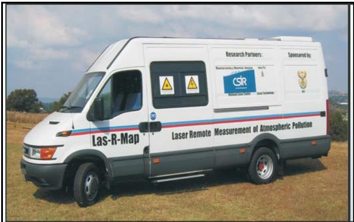
FIGURE 2.2: CSIR mobile LiDAR van (adopted from Sharma, et al., 2009).
