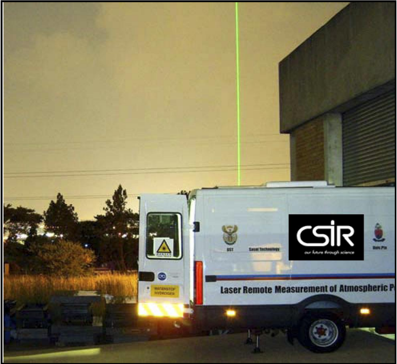
FIGURE 3.5: NLC-CSIR-Mobile LIDAR system.
