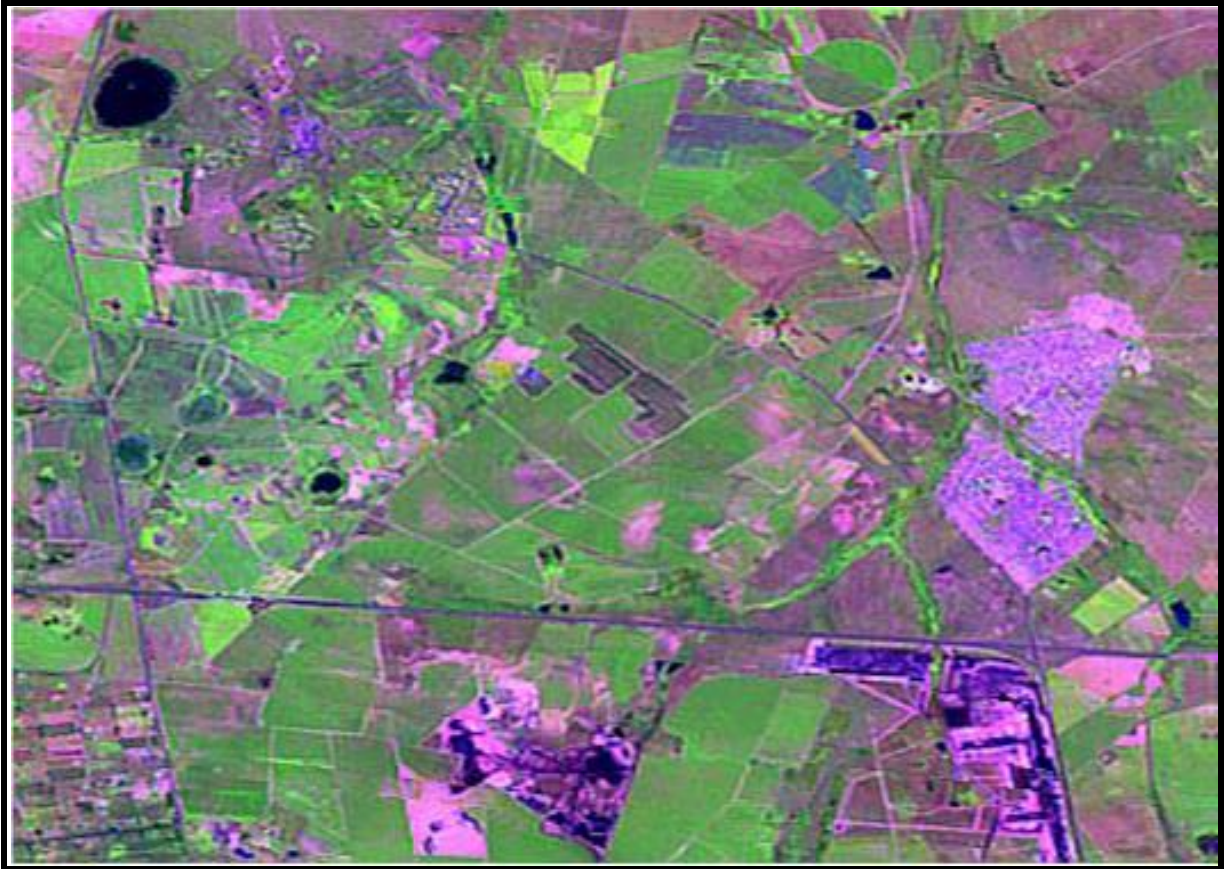
FIGURE 3.1: Surface heterogeneity over Highveld region detected using normalized digital vegetation index (NDVI) for the tile e29s26 obtained by the Landsat platform 7 with the sensor ETM+ at 03 July 2006. Pixel size – 30 m. The size of the shown area is 20.6 km by 20.6 km. Data source is FAO FRA Landsat Imagery Database http://globalmonitoring.sdstate.edu/projects/fao/index.html .
