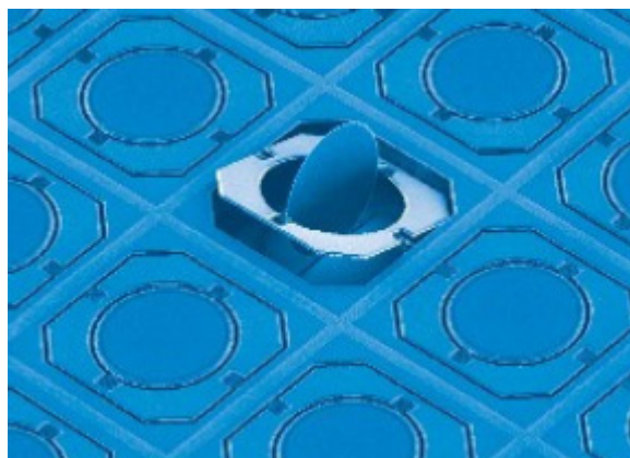
Figure 2.12: 3D MEMS cross-connect in two different states [20].
