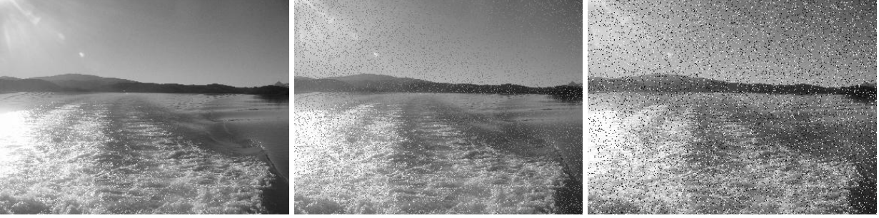
Fig. 2: Illustration of impulse noise ( N(127, 100) ) (center) and salt-and-pepper noise (right). The parameters used were \alpha = 0.5 and p = 0.1 .
