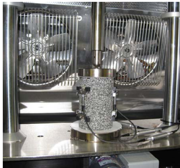
(b) Instrumentation of test specimen
