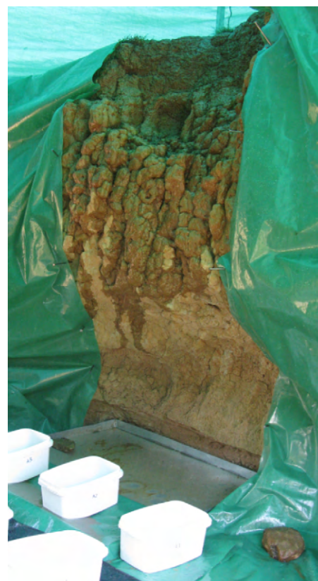
Fig. 3. Rainfall simulation along a 1 m width and 2.3 m in height. Position of some of the twelve 0.27 m × 0.17 m buckets for splash collection and of the microplot to gather both the vertical runoff and the entire soil aggregates falling down the bank. Picture taken 6 min after the beginning of a 45 min and 60 mm h -1 intensity artificial rainfall with the sprinkler for rainfall simulation located at the vertical of the bank.
